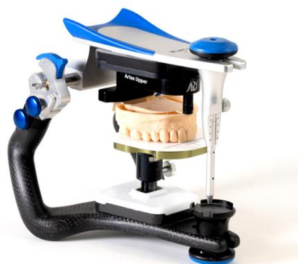
**FIGURE 24** — Printed Upper Model on Platform
